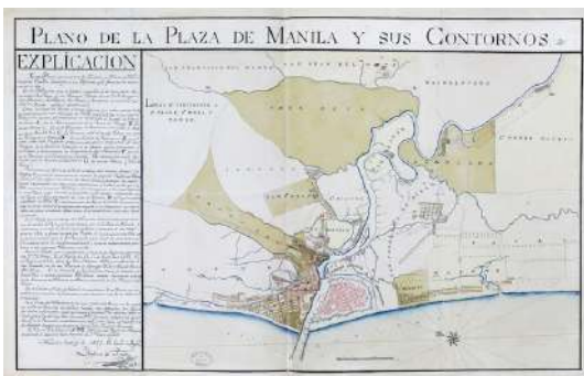
Plan of the square of Manila and its environs, with the dike built to neutralise the progressive silting up of the river port at the mouth of the Pasig River. 4 January 1814. Idefonso de Aragón y Abollado, commander engineer (1760 - ?). Facsimile reproduction. General Archive of the Indies, Seville, Spain. MP - Filipinas, 133.
