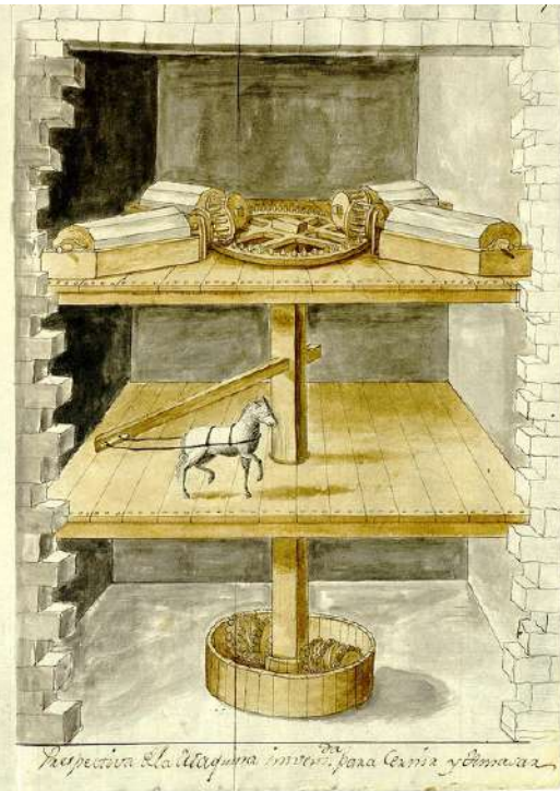
Perspective of the machine for sifting flour and kneading bread, invented by Francisco Antonio de Horcasitas, in Mexico. 1786. Facsimile reproduction. General Archive of the Indies, Seville, Spain. MP - Ingenios, 193.
